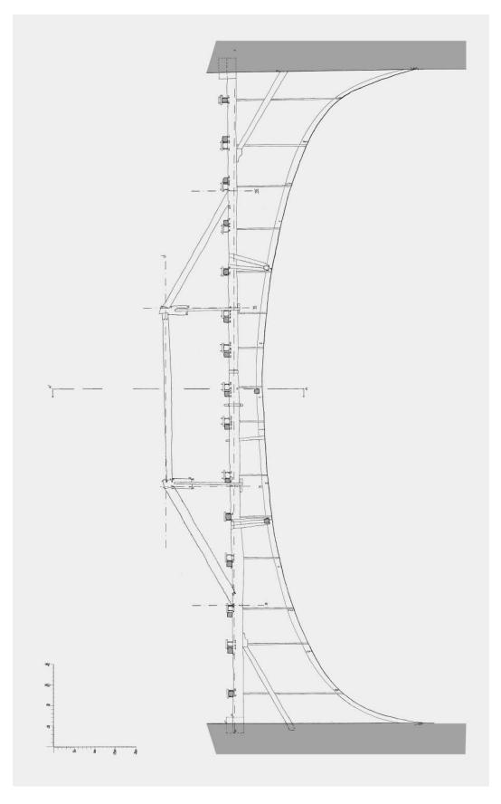
**Fig. 7:** Rome, S. Pietro in vincoli: detail of the structure holding the wooden vaults. (Drawing by the author.)
