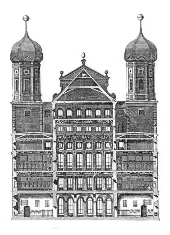
**Fig. 4:** Augsburg Town Hall: cross section with roof and ceiling structure (after the engraving by Salomon Kleiner, 1733; Baum 1908, Tav. VIII, Fig. 11, Detail).
